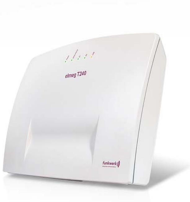
The settings are transferred to the PBX via the USB port and your PC can surf the Internet by ISDN directly on the USB port via the PBX. The shipped TAPI and CAPI drivers serve to implement Computer Telephony Integration (CTI) in a simple way.
